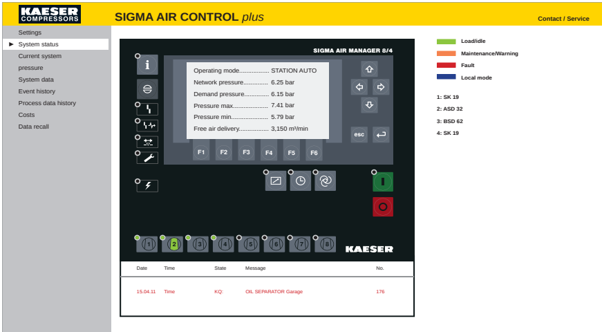
Fig. 5c: Overview: Control and management system
