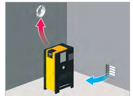
Fig. 2: Forced ventilation with extractor fan for compressors from 5.5 to 11 kW
